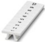
Zack marker strip, Strip, white, labeled, printed horizontally: consecutive numbers 1 ... 10, 11 ... 20, etc. up to 91 ... 100, mounting type: snap into tall marker groove, for terminal block width: 3.5 mm, lettering field size: 3.5 x 10.5 mm, Number of individual labels: 10
