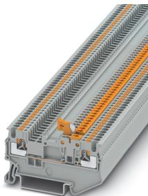
Knife disconnect terminal block, nom. voltage: 400 V, nominal current: 10 A, 1 level, connection method: Push-in connection, Rated cross section: 1.5 mm<sup>2</sup>, cross section: 0.14 mm<sup>2</sup> - 1.5 mm<sup>2</sup>, mounting: NS 35/7,5, NS 35/15, color: gray
